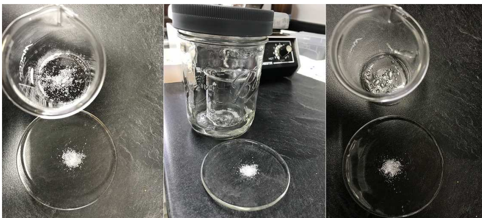
Figure 6.1: Sodium acetate trihydrate spoilage test. The photo on the left shows sodium acetate trihydrate crystals in a beaker and on a watch glass. The beaker was closed in a Mason jar with water on the bottom of the jar overnight (center photo). The next morning (right photo), the crystals on the watch glass were the same, but the crystals in the beaker had become water droplets.
