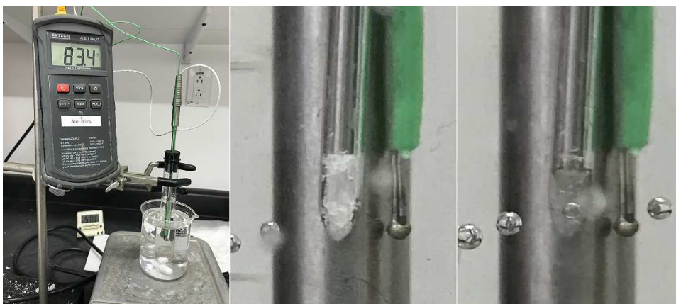
Figure 6.2: Melting point apparatus (left photo). A few milligrams of solid sample in a glass capillary next to a thermocouple (green wire) in a temperature bath on a hot plate stirrer are observed for melting as the temperature of the bath slowly increases. The thermocouple temperature display is showing 83.4°F near the beginning of a measurement. The two close-ups show the thermocouple bead and the glass capillary with the solid sample shortly before (center) and shortly after (right) beginning to melt.
